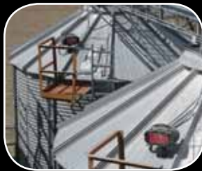
Measuring corn in a grain storage silo.
