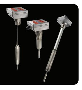
piezoelectric system, which gets electrical pulses from the electronics. These electric pulses enlarge the size of the piezos which leads to a bowing of the rod. Since the pulses are exactly on the frequency where the rod is in resonance, the whole rod starts swinging. A second piezo electric system works as a swinging detector. If the piezo gets distorted, it gives a voltage signal to the electronics. This way, the electronics can check if the rod is vibrating or not.
