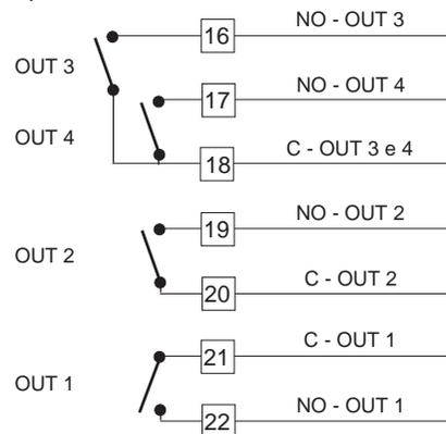
Fig. 9 RACCORDEMENT DES SORTIES A RELAIS
