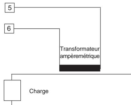
Fig. 8 RACCORDEMENT DU TRANSFORMATEUR AMPEREMETRIQUE
