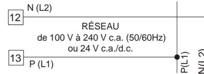
Fig. 4 RACCORDEMENT A L'ALIMENTATION
