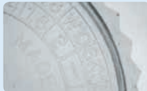
Direct Backlight (MDBL-CB70) Ordinary light transmitted evenly through the entire object.
