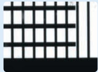
Electrodes on Liquid Crystal Glass MEBL-CW7050
