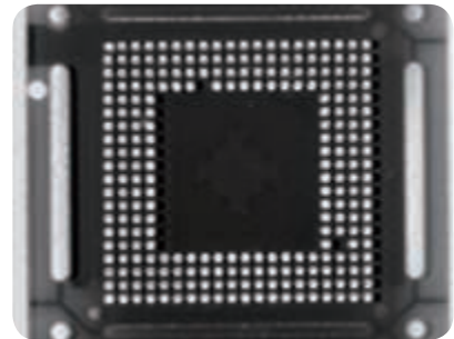
Actual image of BGA (Ball Grid Array) chip illuminated by a Darkfield ringlight clearly identifies where solder balls are missing.
