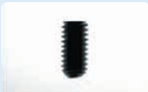
Direct Backlight (MDBL-CB70) Shape unclear because of stray, direct light.
